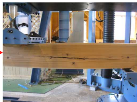
Fig. 5.2 The span condition of short beam shear test by asymmetric four-point loading method
